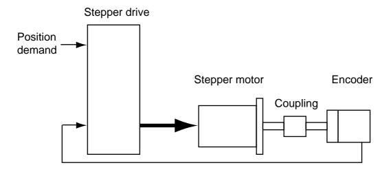
Figure 4-12. Closed Loop Operation
